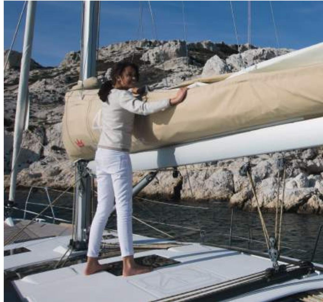
Inclined boom for easy packing
